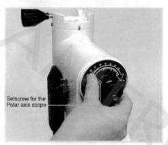
③ Screw the SX Polar axis scope into the Polar axis of the mount by gripping about the setscrew as a holding aid.
