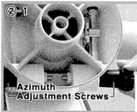
Place the equatorial mount on the tripod head as shown in the Figure, and fix it with the fixing knob from beneath.
