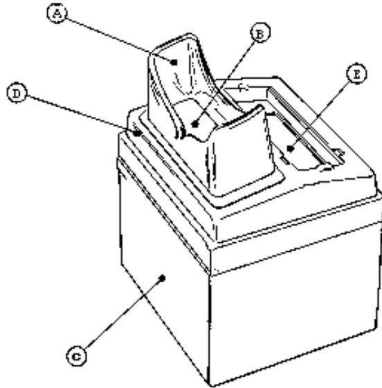
1. Lift flexible eyepiece (A) and cover assembly (B) out through top of cabinet.
