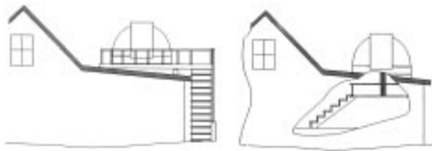
ON ROOF IN ROOF FIGURE 2.3
