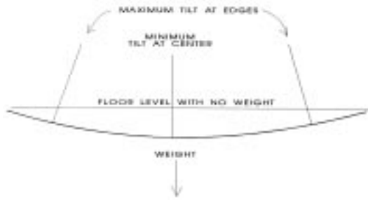
FLOOR, ROOF TILT FROM PERSON FIGURE 6.4
