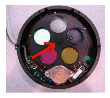
3. The rubber caps plugging the screw holes in the CFW-8A need to be pushed out next.
