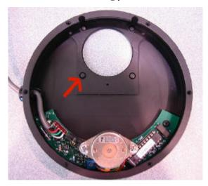
4. Use a blunt non-marring tool to avoid scratching the anodized surfaces. The caps are easiest to push out from the back of the CFW-8A as shown in the image:
