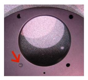
5. Remove the D-Block unit from the front of the camera head by removing the 4 phillips head screws. Put the D-block and screws in a safe location, you may need to use them later to attach optional accessories like the AO-7.
