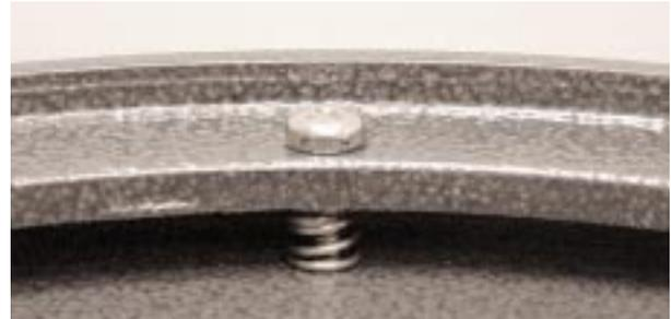
**Figure 18.** The primary mirror collimation screws are the ones with the springs visible just under the mirror cell casting.
