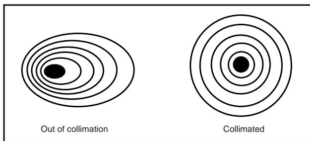
**Figure 16.** A star test will determine if a telescope's optics are properly collimated. An unfocused view of a bright star through the eyepiece should appear as illustrated on right if optics are perfectly collimated. If circle is unsymmetrical, as in illustration on left, scope needs collimation.
