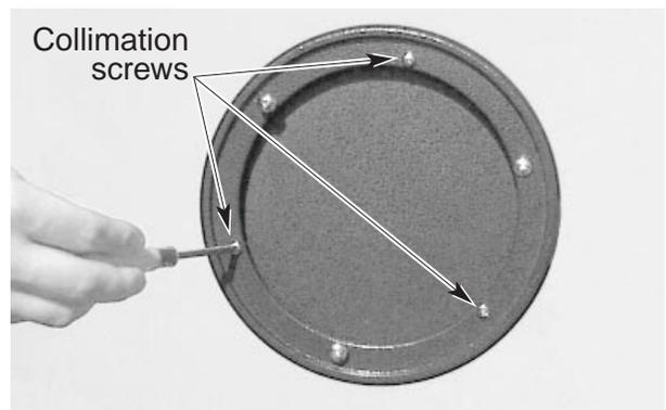
**Figure 20.** The tilt of the primary mirror is adjusted by turning one or more of the three spring-loaded collimation screws.
