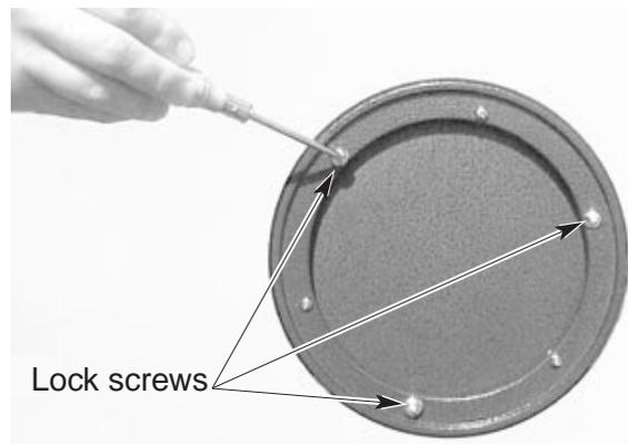
**Figure 19.** The three screws that lock the primary mirror in place must first be loosened before any adjustments can be made.
