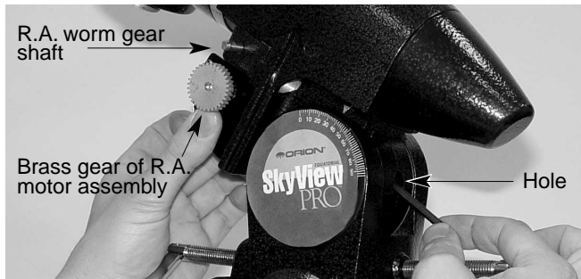
Figure 3. The motor is attached to the front of the mount by a socket head cap screw pushed up through the hole in the rear of the mount.
