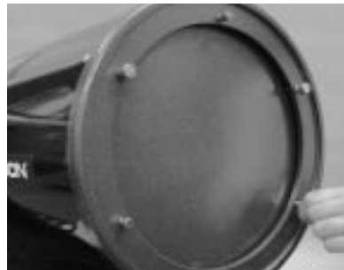
Figure 17: The three thumb screws that lock the primary mirror in place must first be loosened before any adjustments can be made.
