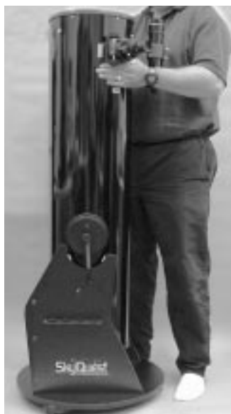
Figure 5. Set the optical tube on the "cradle" of the base so that the altitude side bearings on the tube rest on the white plastic "pads."
