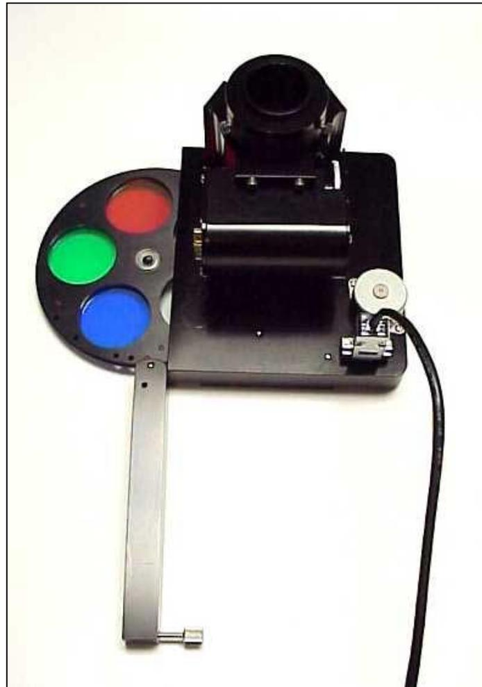
*Figure 3-4. IFW with Door Open for Wheel Change
