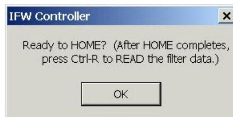
Be sure to perform a Read after the Home has completed by pressing control-R or selecting "Read" from the Config pull-down menu.
