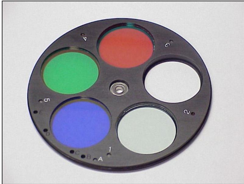
Figure 3-2. 5-Position Filter Wheel with RGB-IR and Luminance filters.
