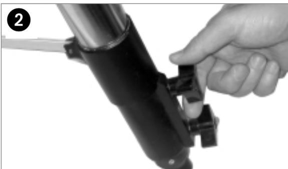
2. Thread in two lock-knobs on each leg (six total) near the foot of each tripod leg. Use the lock-knobs to vary the height of the inner, extendible tripod leg sections. Tighten the locks to a firm feel only; do not overtighten.
