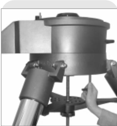
Fig. 48: Attach the drive base to the tripod.
