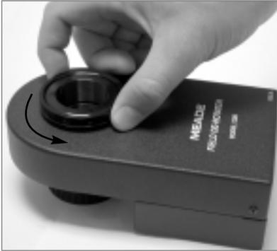
*Fig. 54: Back off the adapter ring one full revolution.*
