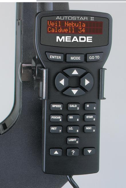
**Control Panel Functions:** Use the telescope's control panel for direct connection of CCD imagers and auto-guiders (*pp. 82 - 97*); plug in an illuminated reticle eyepiece for photo-guiding, adjusting reticle brightness from the Autostar II handbox; or power the standard-equipment Zero Image-Shift Microfocuser. Two RS-232
