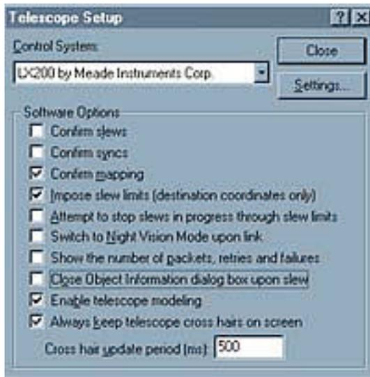
You may also use the "The Sky's" Telescope->Options->Initialize menu for setting up date, time, and location of your observing site. All values will be set permanently and stored into SRAM and/or RTC. It is best to use the items from bottom to top.
