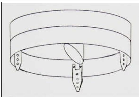
**Nose assembly showing adjustable focal-point system**
