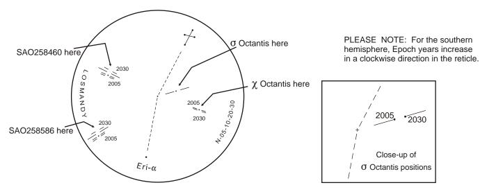
This diagram shows only the reticle lines used for Southern Hemisphere alignment. The 2 sets of lines for χ Octantis represent the Epochs 2005 and 2030. The 4 sets of lines for SAO258460 and SAO258586 represent the Epochs 2005, 2010, 2020 and 2030. The gap in the longest line is for 2020, the 2 gaps on the 2 segments counter-clockwise are for 2010 and 2005, and the remaining gap clockwise is for 2030. The stars are diagramed in their Epoch 2010 positions.
