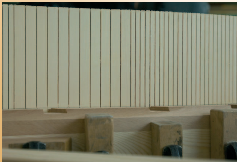
In producing the outer rim's curvature, bending the solid wood is made possible via selective incisions.
