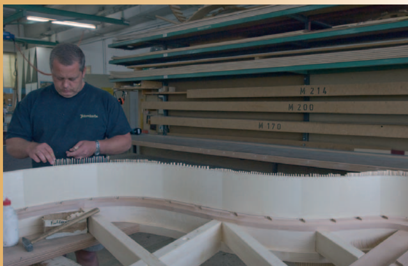
In order to fill in the incisions once again, spruce wedges are inserted into the top side of the outer rim.
