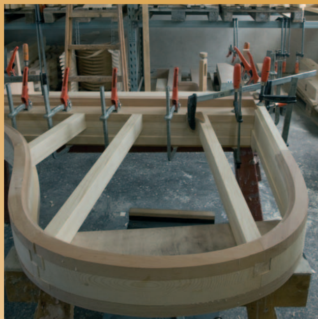
In a genuine Bösendorfer, the sub-frame is produced from resonating spruce and copper beech.
